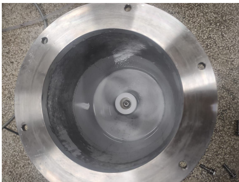
Figure 11 – Empty and clean chamber before irradiation.
