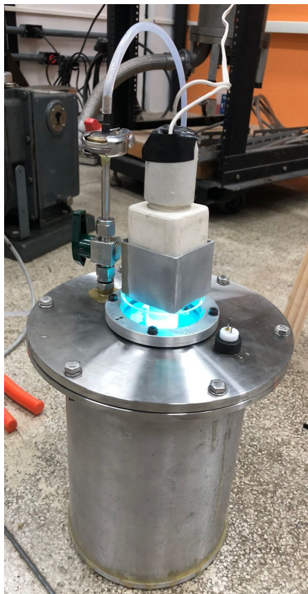
Figure 9 – Sealed irradiation chamber coupled to a vacuum pump, with a UV-C lamp irradiating a water sample.
