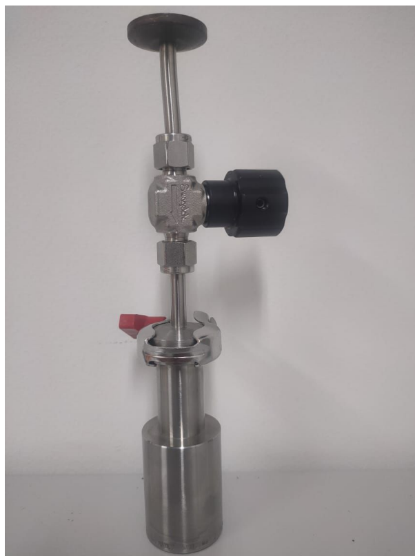
Figure 10 – Portable chamber responsible for the storage and transport of H_2 produced in water radiolysis.
